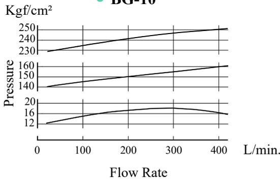
**Min. Adj Pressure & Vent Pressure Vs Flow**
