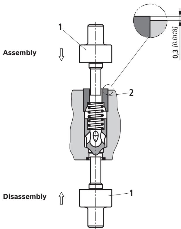
Disassembly/assembly without any damage is ensured by using the special multi-purpose tool (1) (material no. **R901182853**, ordered separately).
