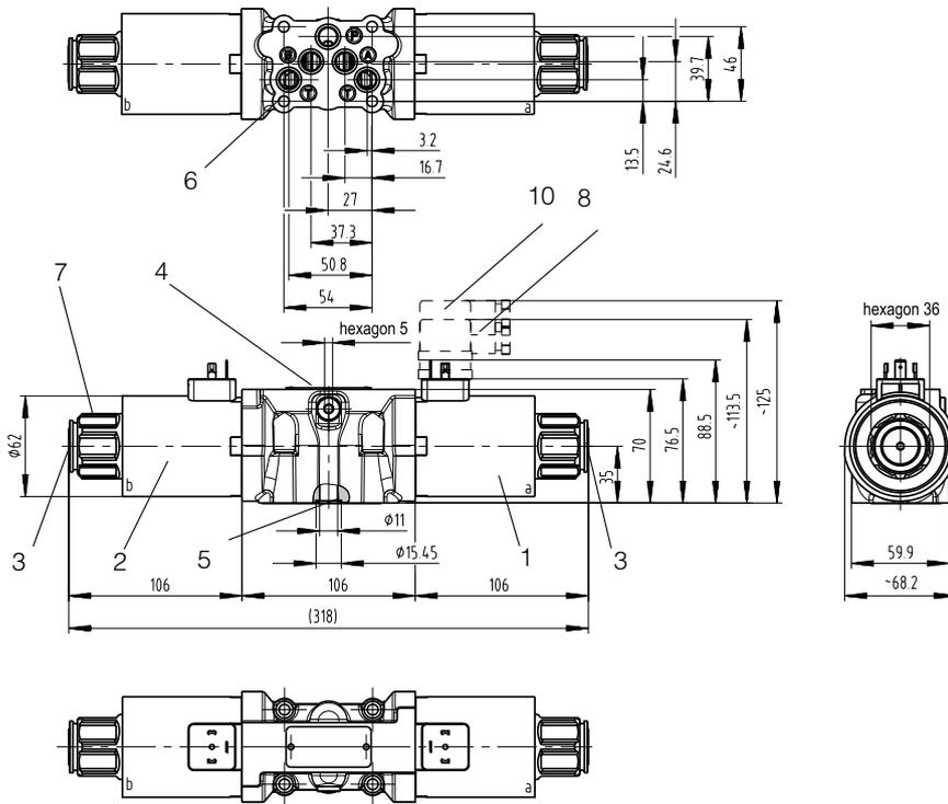
All valves HD5-ES-\* conform with ISO and CETOP specifications for mounting surface dimensions and for valves height.
