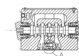
and are kept sealed on the P port of the valve by an OR of 9,25x1,78 mm sizes (example OR 110-2037)
