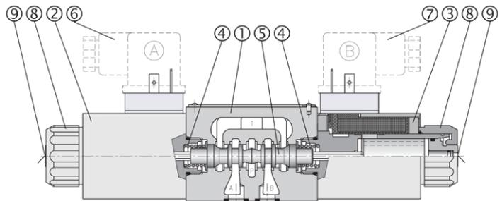
The spool 5 shifts into the valve body 1 subject to the action of springs 4 and solenoids 2. Spool 5, depending from its shape and its position in the valve body, opens and/ or closes passages between P, A, B and T ports, thus controlling the direction of the hydraulic flow.
