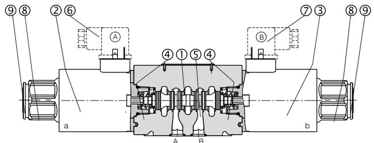
The spool 1 shifts into the valve body 7 subject to the action of springs and solenoids 2 and 3. Spool 1, depending from its shape and its position in the valve body 7, opens and/or closes passages between P, A, B and T ports, thus controlling the direction of the hydraulic flow. In case of electric cut-offs the spool can be manually shifted by acting on the override pins 9, located at the end of the solenoids and accessible through the retaining nuts.
